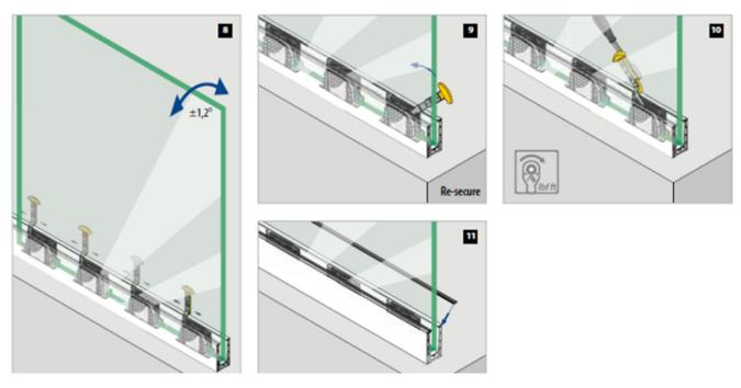
FIGURE 3 (CONT'D)—GUARD RAIL ASSEMBLY COMPONENTS (Q-DISK SYSTEM)
