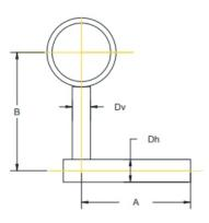
FIGURE 1—ADJUSTABLE HANDRAIL BRACKET
